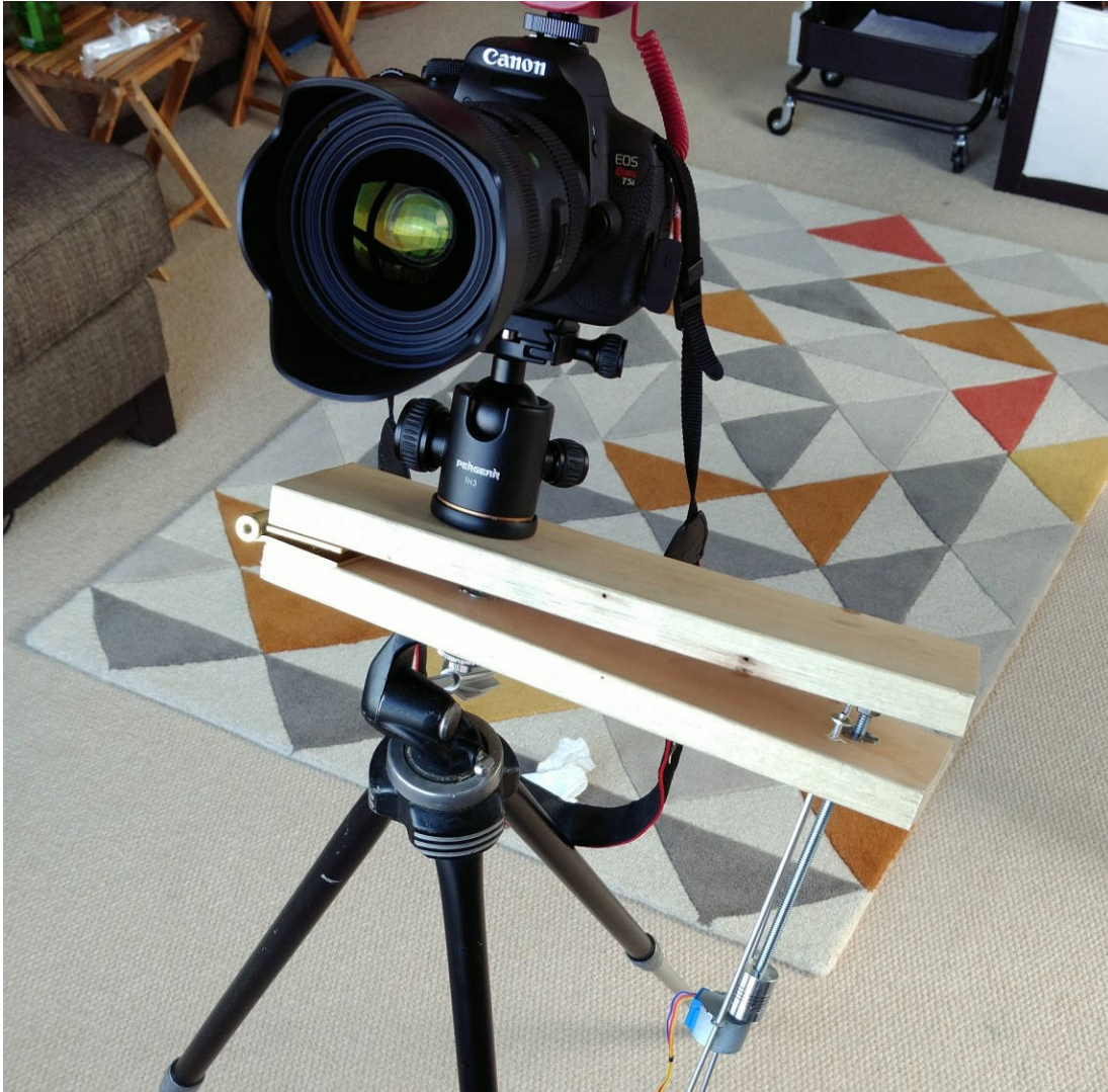
Figure5: A photo of a working star-tracking camera mount.
